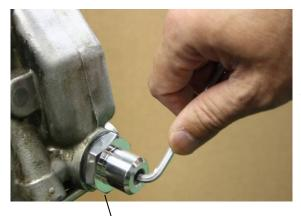
With a gasket, please perform clamping by designated clamping torque. Please relax the Adjust bolt not to take tension.
